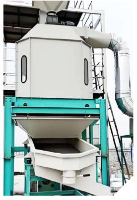
Cooling & screening combined Counterflow cooling Moisture removal
