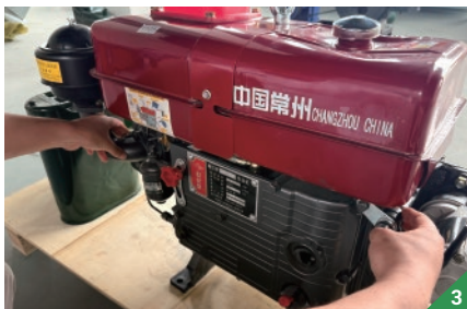
Hold down the decompression lever and start the engine
