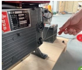
Measuring Oil Level with the Dipstick
