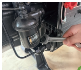
Loosen the Fuel Injection Pump Air Bleed Screw to Vent All Air
