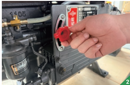
Move the control lever to the START position
