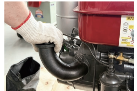
2. Blocking the Air Intake Pipe
