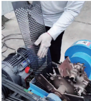
Insert the new screen along the inner wall of the screen groove
